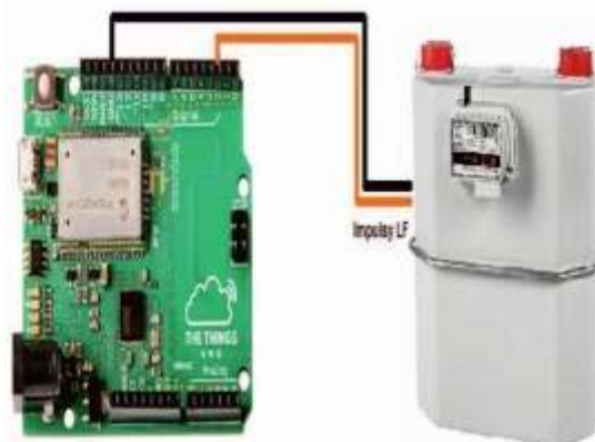
Fig. 2. Gas meter connection with the TTN-UNO868 system
